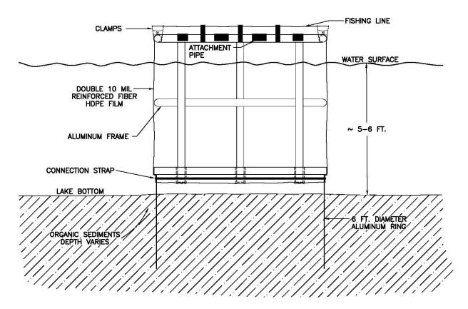
Figure 3-2. Typical Isolation Chamber Installation.
