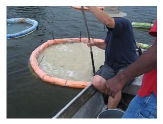
Slurry mixed into chamber with paddle
