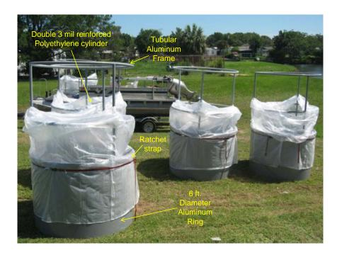
Figure 3-3. Assembled Isolation Chambers Prior to Installation in Silver Lake.
