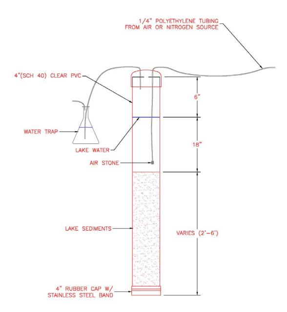
Figure 4-15. Schematic of Sediment Incubation Apparatus.
